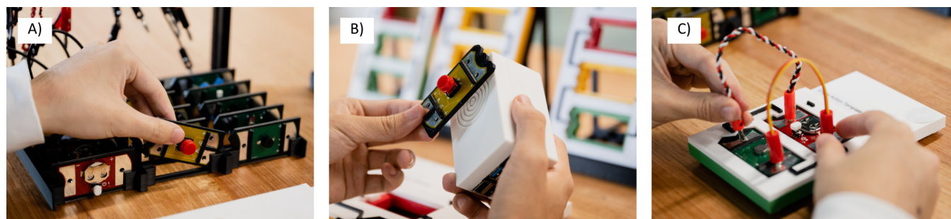
Figure 1: We adapted an existing electronics toolkit with a) a set of 3D printed physically identifiable covers for modular electronic boards, b) a Near Field Communication (NFC) device to provide participants with component-specific audio descriptions and use instructions, and c) self-describing 3D printed circuit templates with tactually distinguishable circuit connectors.
