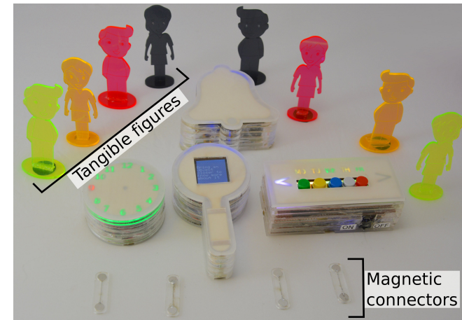
Figure 1: AwareKit consists of six types of tangible modules. Four modules for retrieving availability information (in the center), tangible figures and magnetic connectors. Tangible acrylic figures used to represent individual colleagues and magnetic connectors for communication between modules.
