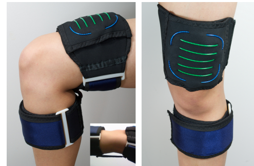
Figure 1. Physical Therapy Prototype for Knee Rehabilitation. Inset shows extended leg with view of the bend sensor.
